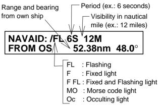
Figure 2-7 Example of buoy, lighthouse data
